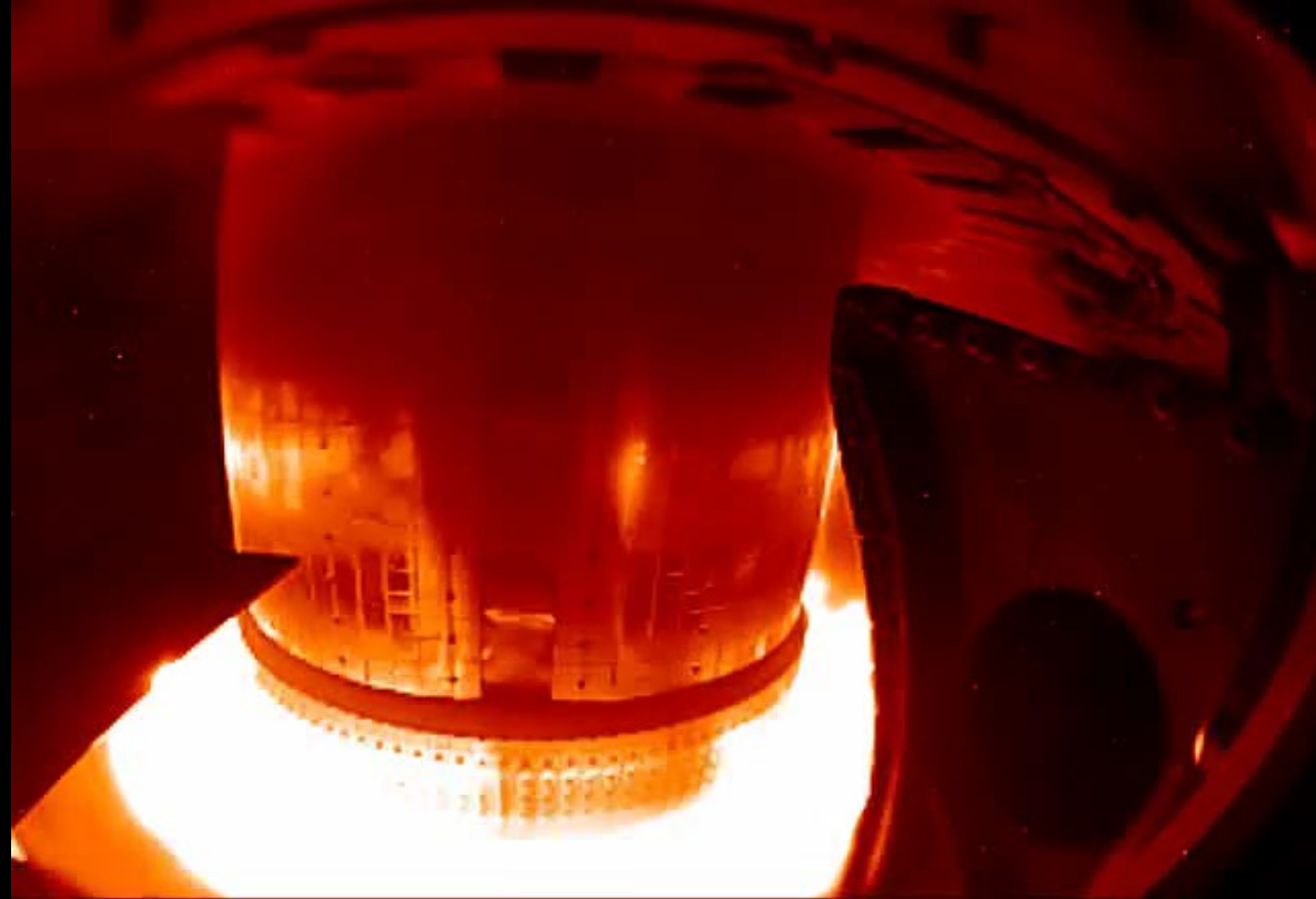
LOSS OF RELATIVISTIC ELECTRONS TO MATERIAL SURFACES VIDEO FROM ALCATOR C-MOD; R. GRANETZ, PRIVATE COMMUNICATION
