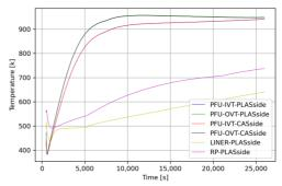
Fig-1: Divertor temperature transients following invessel LOCAs in the cassette and in the target - DEC accident (PFU: Plasma Facing Unit, IVT (OVT): Inner (Outer) Vertical Target, etc.)
