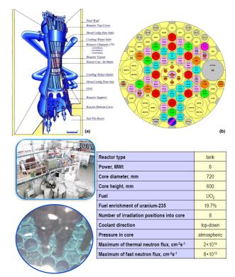
Fig-1: BR-2 and WWR-K reactors
