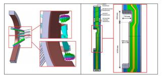
Fig-2: View of the BB COB segment with the integration of the ECH system.
