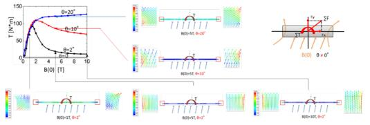
Fig-1: Torque on beam plate by FEM analysis
