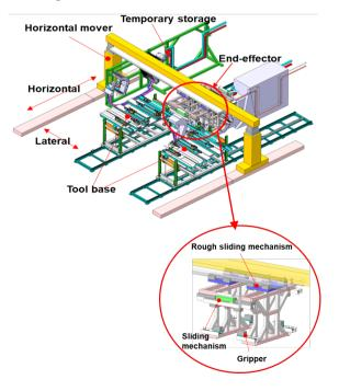
Fig.-2: (Upper) Schematic view for RMS and (Lower) enlarged end-effector
