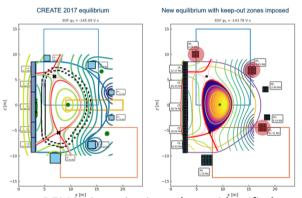
Fig.-1: MHD equilibrium together with configuration of poloidal coils. (left) without/ (right) with keep-out zone applied to poloidal coil positions
