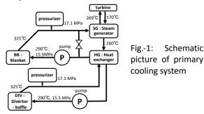
The decay heat of the Breeding Blanket (BB) can be removed by natural convection as long as the heat removal capacity on the steam generator side is operating. To remove the decay heat of the divertorbaffle, it is necessary to operate the pumps in the cooling line. Redundancy is required for pumps in the SG and divertor-baffle cooling line.
