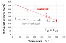
Fig.-2: Neutron irradiation (~5 dpa) effect on tensile properties of CuCrZr-IG
