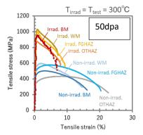
Fig.-1: BM: Base Metal, WM: Weld Metal, FGHAZ: Fine-Grained Heat-Affected Zone, OTHAZ: Over-Tempered HAZ. Like BM, WM and HAZ undergo hardening and loss of ductility by irradiation.
