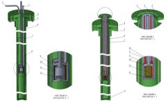
Fig.-1: examples of the design of rig and capsule for in-situ T release measurement in WWR-K; (left) option 1 and (right) option 2 (various options have been investigated by considering effectiveness and precision for measurement).
