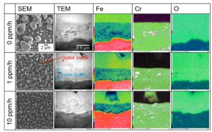
Fig.-1: Effect of H<sub>2</sub>O<sub>2</sub> on corrosion property of F82H
