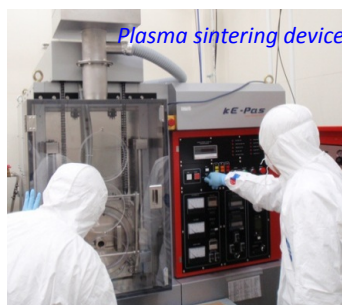
Fig.3 Plasma sintering device and workers handling beryllium with personal protective
