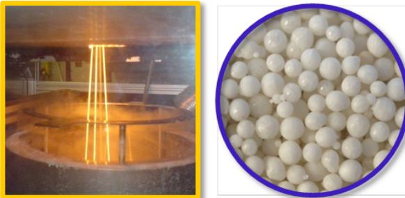
Fig. 1: Pebble fabrication by the melt-based process in an experimental facility (left). Three nozzles are operated simultaneously in this case. Each melt jet consists of individual droplets. The solidified ceramic pebbles exhibit a mean diameter of 700 µm (right).
