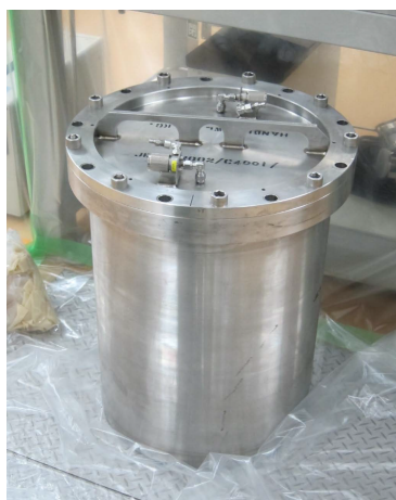
Figure 1. Shipping container for dust sample Dust sample contains 80GBq of tritium and Type A Package was needed for the transportation.
