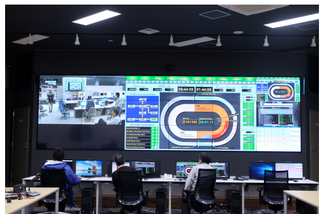
Fig.2 Demonstration of the remote experiment of JT-60SA in the REC room. The status of the discharge and facility were displayed in the large video wall and the video conference.
