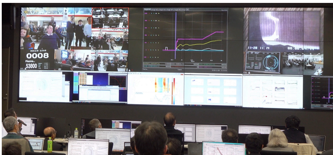
Large video wall in the REC room showing the video conference and countdown (left), the live data of the main plasma parameter (center), the video of the plasma (right), and so on.
