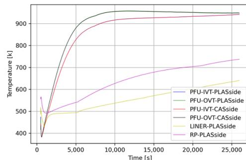
Fig-1: Divertor temperature transients following in-vessel LOCAs in the cassette and in the target – DEC accident (PFU: Plasma Facing Unit, IVT (OVT): Inner (Outer) Vertical Target, etc.)
