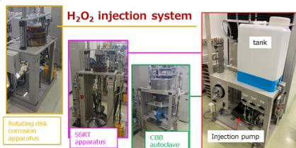
Fig-1: Corrosion test systems with hydrogen peroxide injection apparatus.
