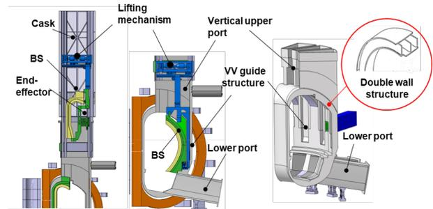
Fig-2: Schematic view for RM for blanket segment (left) and VV configuration (right)
