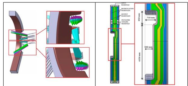
Fig-2: View of the BB COB segment with the integration of the ECH system.
