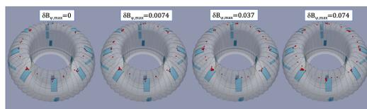
Fig.-3: Collision points of REs with  $E=100\text{MeV}$  in EU DEMO with four different perturbation strengths (DEMO Design Task-1 TROs)
