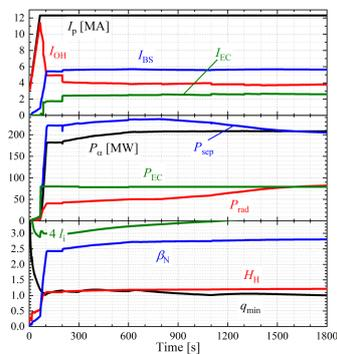
Fig.-1: Pulsed plasma operation scenario using EC only for H&CD in JA DEMO
