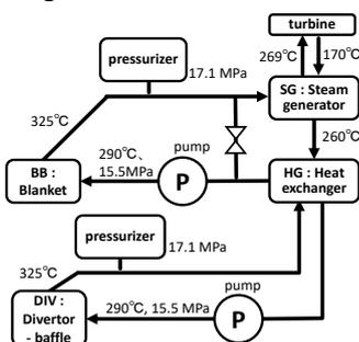
Fig.-1: Schematic picture of primary cooling system
