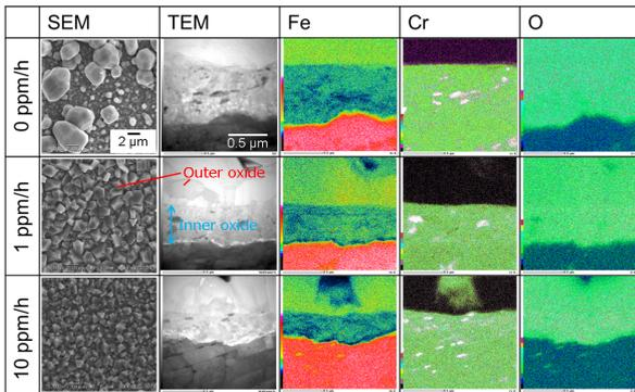
Fig.-1: Effect of H<sub>2</sub>O<sub>2</sub> on corrosion property of F82H
