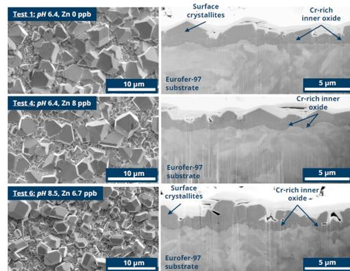
Fig.-2: Effect of Zn addition on water corrosion of EUROFER97
