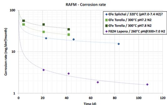
Fig.-3: Corrosion rate of EUROFER97
