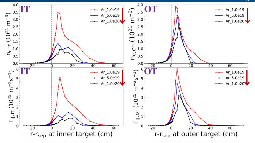
As Ar seeding rate is increased from 1.0e19 atom/s to 1.0e20 atom/s, the electron density and particle flux density at the divertor targets reduced, which shows that divertor enters detachment.
