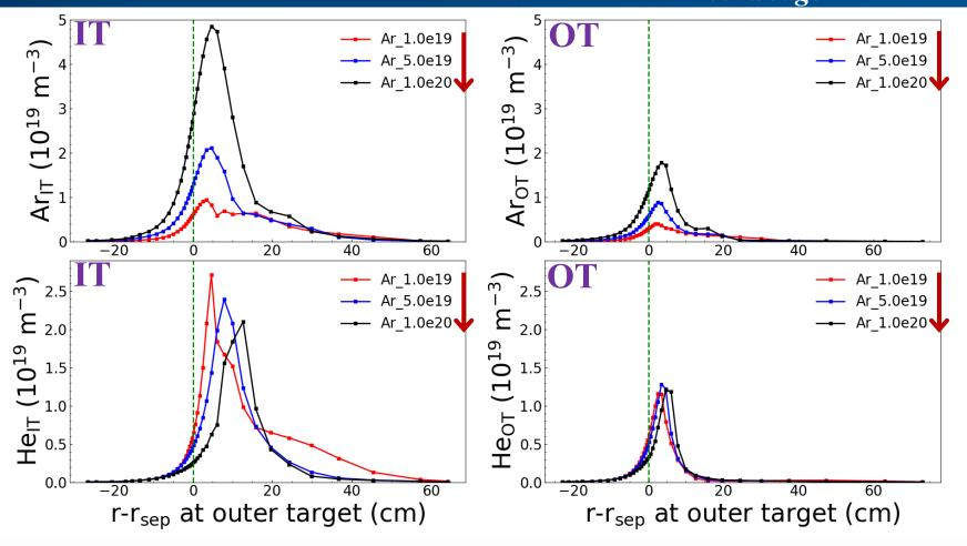
✓ As Ar seeding rate is increased from 1.0e19 atom/s to 1.0e20 atom/s, Ar density are increased at the inner and outer divertor target.
