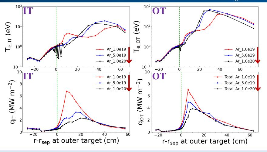
As Ar seeding rate is increased from 1.0e19 atom/s to 1.0e20 atom/s with increasing divertor radiation, the peak heat load at inner and outer divertor target are reduced separately.
