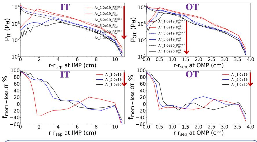
As Ar seeding rate is increased from 1.0e19 atom/s to 1.0e20 atom/s, the momentum loss is extended to outer flux surface.
