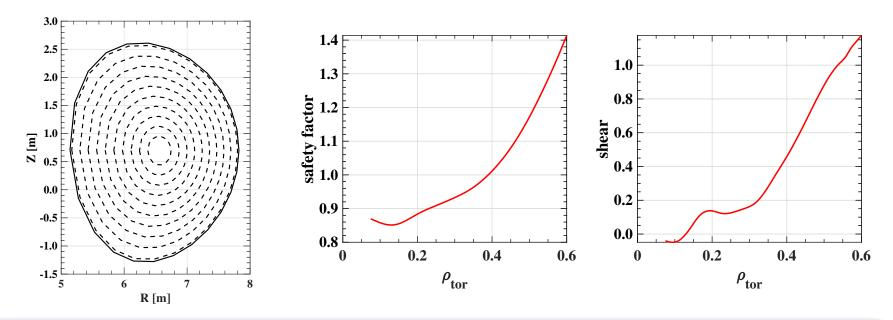
• A relaxed q-profile below q = 1 was chosen to mitigate strong KBM instability observed with a flat q-profile.
