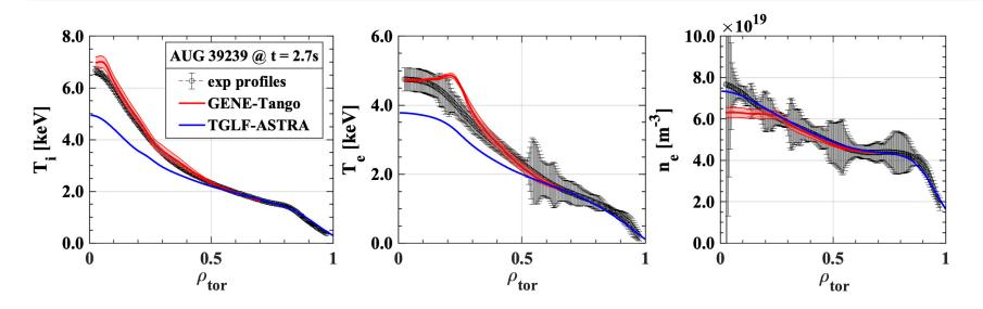
• Experimental  $T_i$  matched only when fast particles and electromagnetic effects are simultaneously retained in the modelling.
