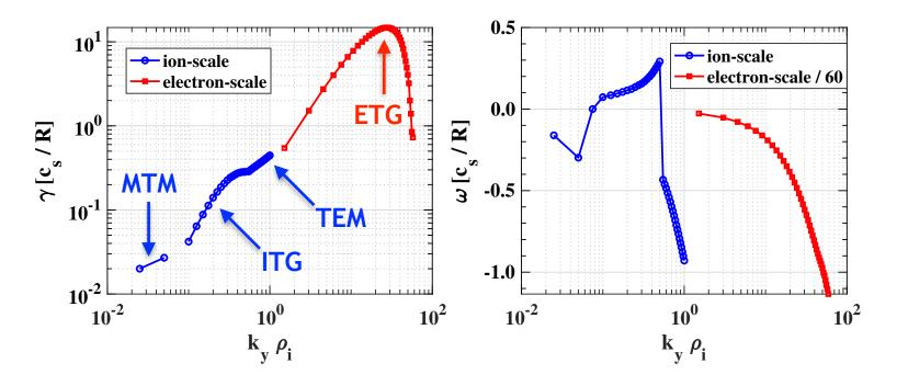
• When computing the ratio  $\frac{\gamma_{ETG}/k_{y|ETG}}{\gamma_{ITG}/k_{y|ITG}} \approx 0.87$  suggesting ETG could be important.
