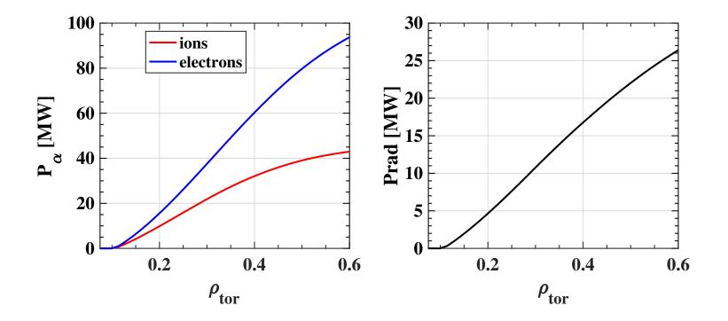
• According to GENE-Tango, total alpha heating power is  $\approx 130 \text{MW}$  with radiation of  $\approx 25 \text{MW}$ .
