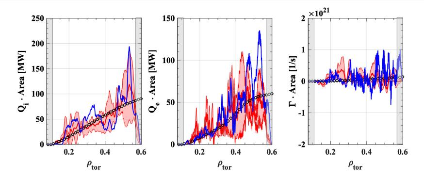
• Using the final GENE-Tango plasma profiles, a stand-alone GENE simulation produces fluxes that align with the power balance.
