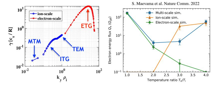
When computing the ratio  $\frac{\gamma_{ETG}/k_{y|ETG}}{\gamma_{ITG}/k_{y|ITG}} \approx 0.87$  suggesting ETG could be important.
